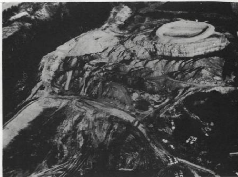
Figure 11 - Aerial view of treatment facility at Shannopin No. 1 air shaft, showing holding lagoon (top), mine pit lagoon (middle) and diked lagoon (bottom).
